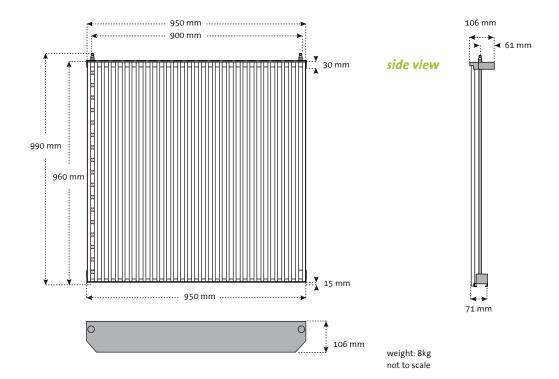
The **Phantom system** consists of two or more frames and ...
