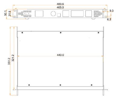
Tolerance: ±0.3 Unit: mm
