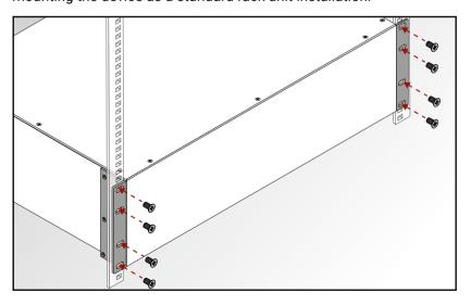
**ATTENTION!** Always use all the four screws for fixing the rack shelf ears to the rack rail. Choose properly sized screws for mounting. Keep minimum two thread left after the nut screw.
