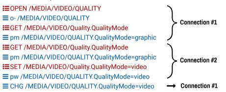
**Explanation:** The first user (**Connection #1**) set a subscription to a node. Later the other user (**Connection #2**) made a change, and thanks for the subscription, the first user got a notification about the change.
