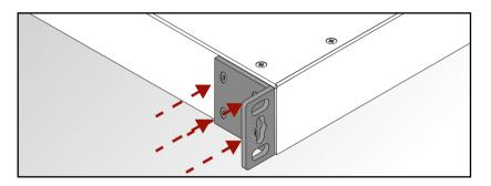
WARNING! M4x8 size is the longest allowed screw for fixing the ears to the housing. A longer screw may touch internal parts.
