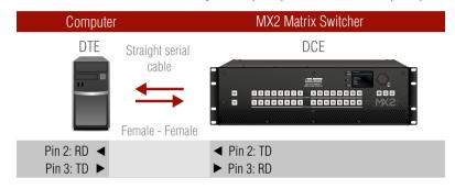
RS-232 Connection Example between a Controller System and a Matrix Switcher
