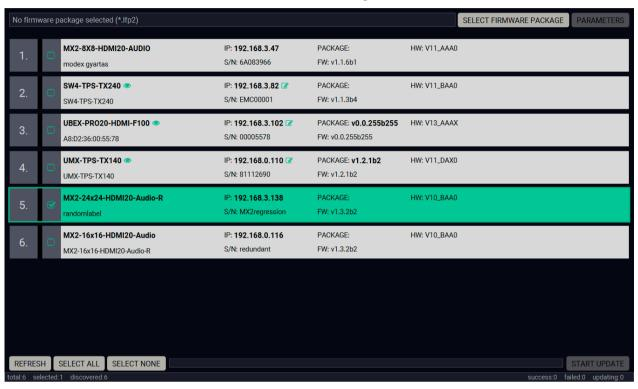
**Step 2.** Select the firmware package file (\*.lfp2). When the file is selected the release note is displayed in the right window. Please read it carefully.
