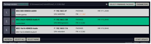
**Step 5.** After the part of LDU2 software upgrade process is finished, the matrix starts the self-upgrade procedure. It is an automatic action and no any user interruption is needed during the operation (the crosspoint buttons show the status of the process).
