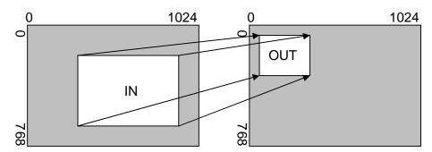
In the example above, 'In' has been set to 300,150 as its top-left source coordinate, with a size of 750,400. 'Out' has been set to 50,50 (i.e. close to the top left) with a size of 250,300.
