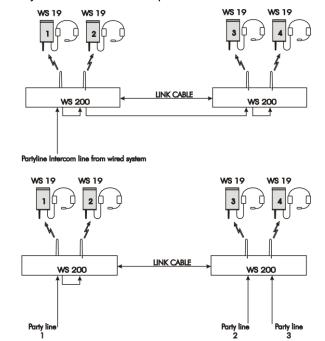
For connecting base station TX/RX modules via their XLR-3 male and female connectors on the rear panels (see drawings above), use short microphone cables.
